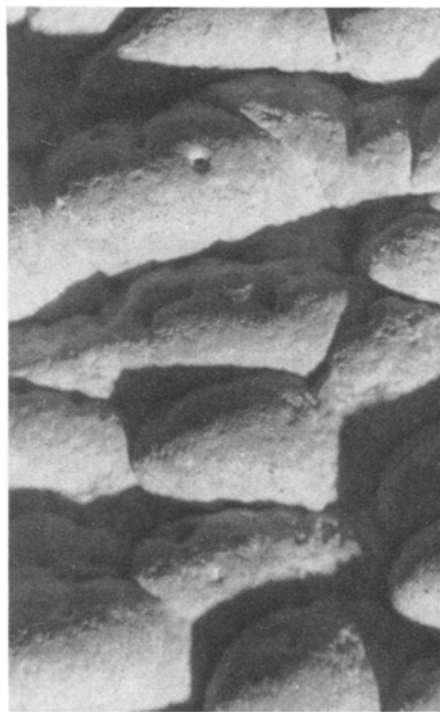
Fig. 5. Deposit from LCJ process pilot plant feed solution in a zinc plant cell under conditions recommended from small scale tests. (Figure width = 5 mm.)
